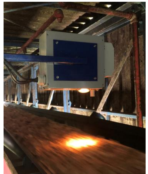
Figure 1: FITNIR MC sensor head over the conveyor.
