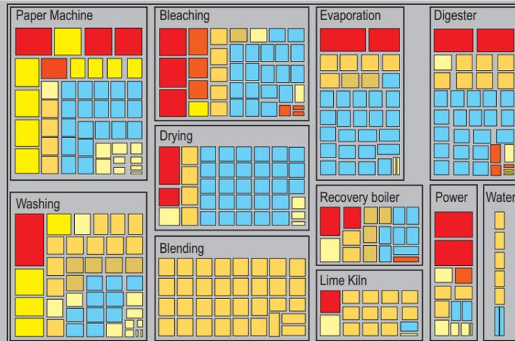
Through systematic analysis, CONTROLSuite identifies the root causes of loop issues. By offering clear, immediate visualisation of all the loops, CONTROLSuite prioritises which loops need to be improved first in order to have the highest impact on overall performance.
