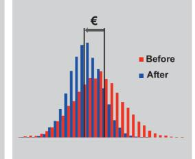
Strength is one of the most important quality parameters in liner and fluting production. **SurfMAX** permits to reduce the variability of the strength, and consequently the strength target can be reduced, leading to major benefits.
