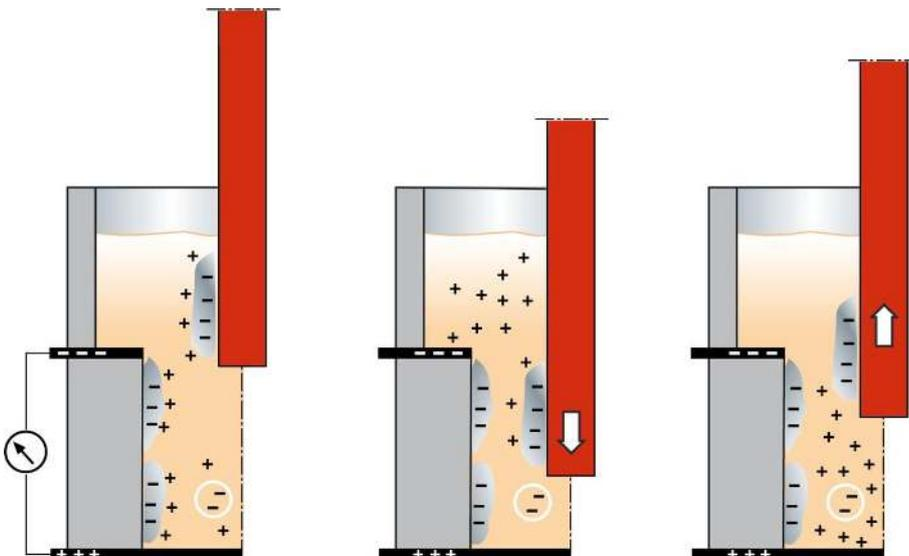
Fig. 2: Schematic of a PCD measuring cell with oscillating piston movement
