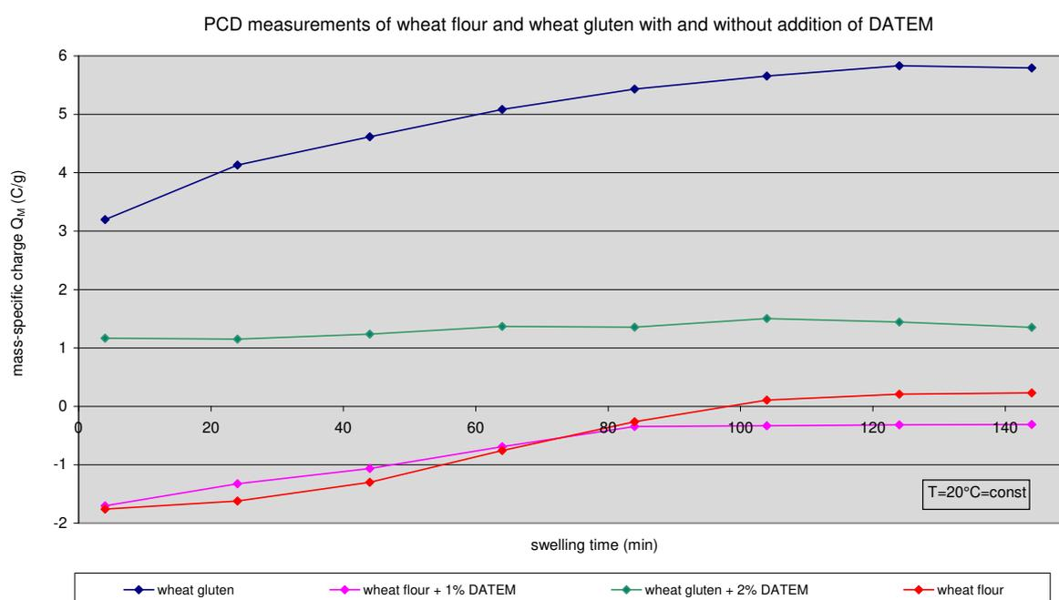
Fig. 6: PCD measurements of wheat flour and wheat gluten with and without addition of DATEM (mass-specific charge  $Q_M$ )
