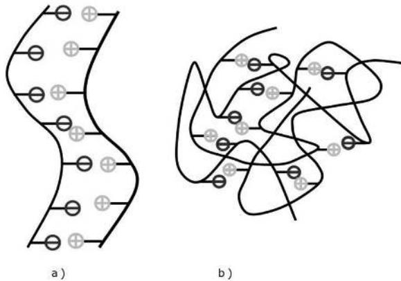
Fig. 3: Symplexing models: (a) ladder model (b) scrambled-egg model
