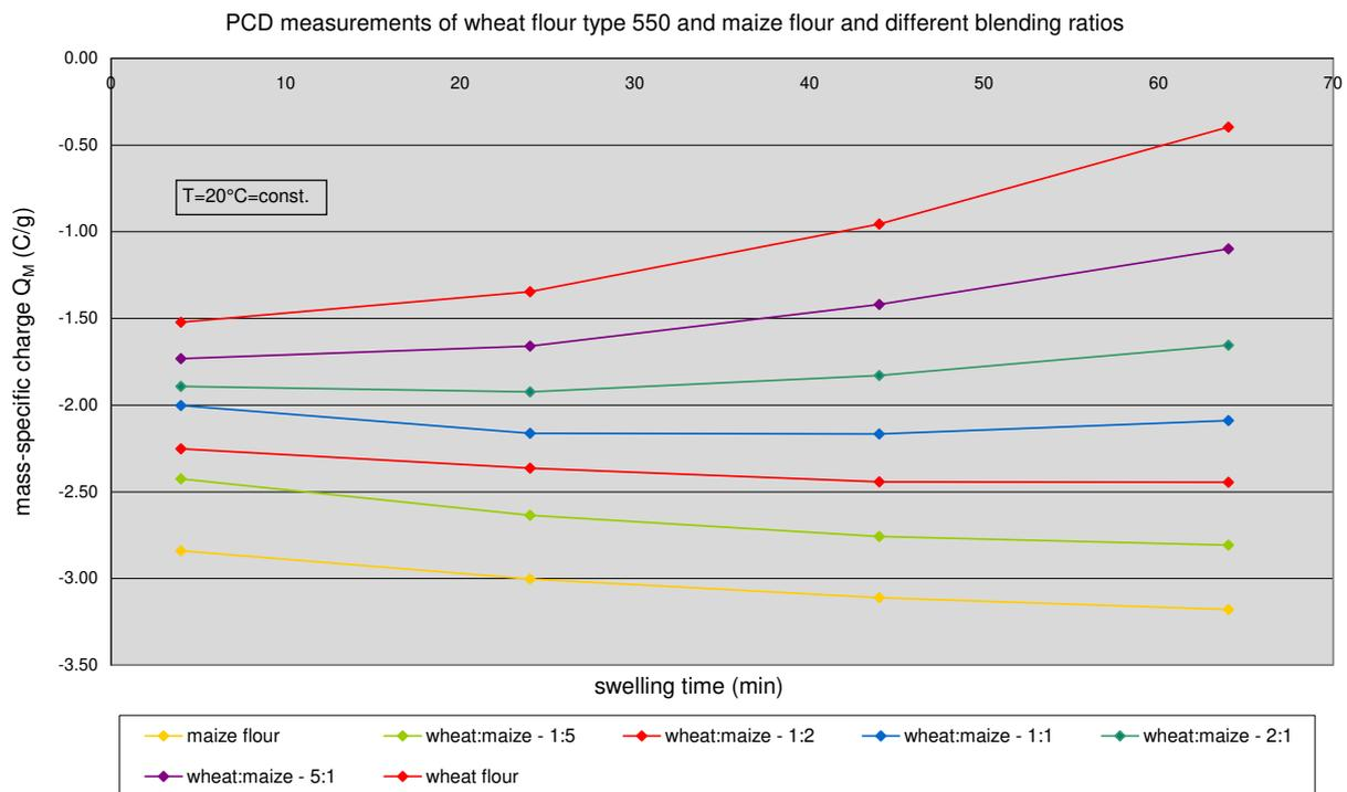
Fig. 5: PCD measurements of wheat flour type 550 (harvested in 2007) with maize flour added at different blending ratios (mass-specific charge  $Q_M$ )
