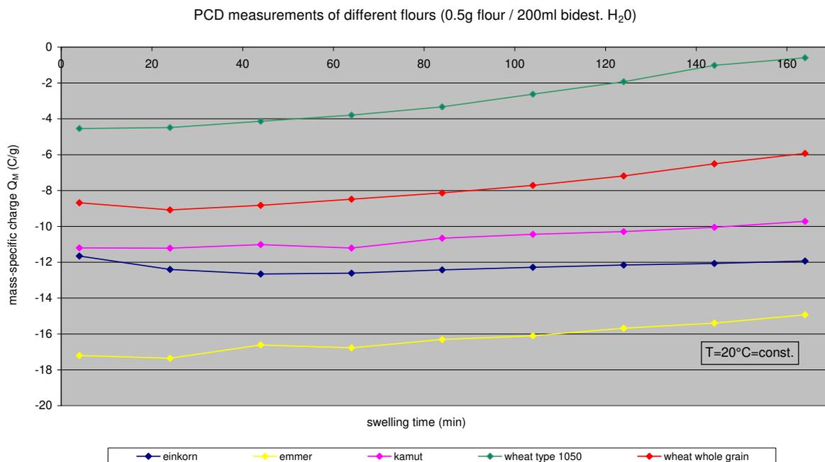
Fig. 4: PCD measurements of different flours (mass-specific charge  $Q_M$ )
