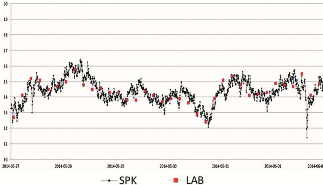
Figure 2: Accuracy of SPK-5500 compared to laboratory kappa measurement
