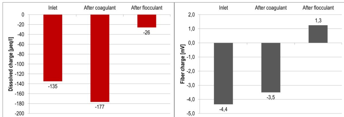
Figure 2: Charge household measured with PCD (red) and SZP (grey)
