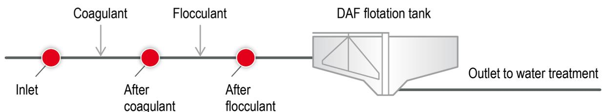
Figure 1: Simplified process diagram
